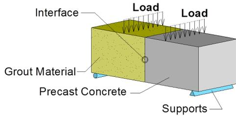
Figure 3. Splitting cylinder test for characterizing bond between precast concrete and field-cast connection grouts.
