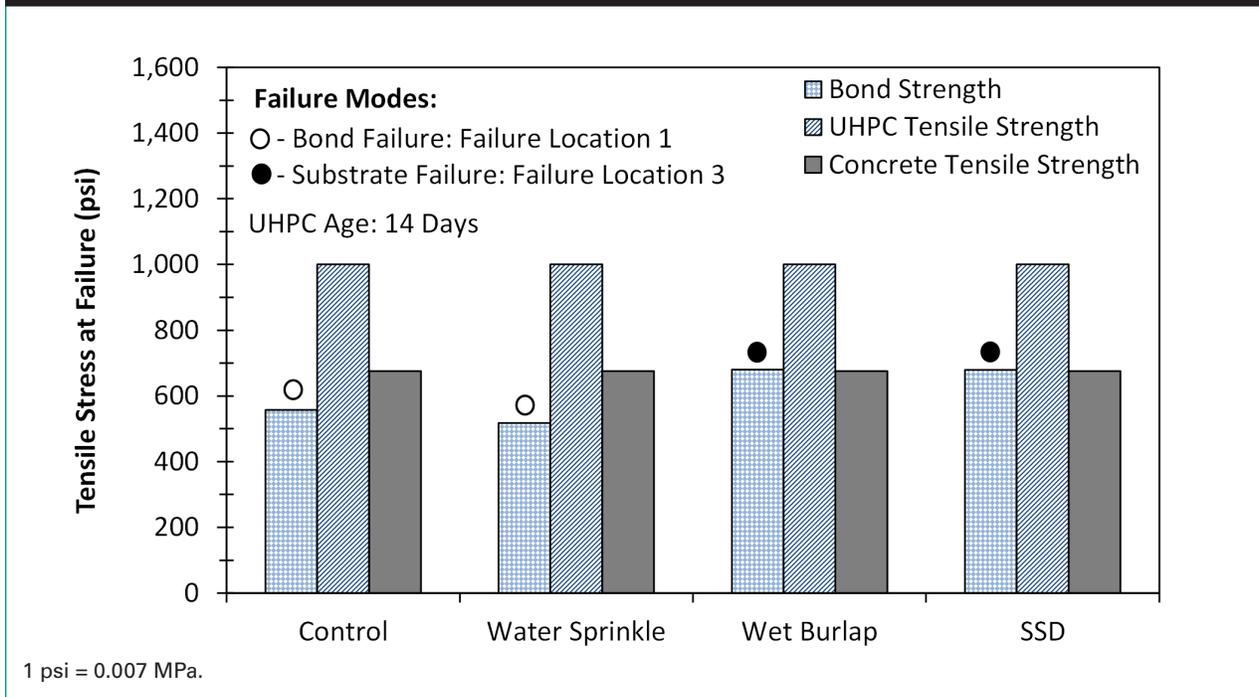
and SSD conditions enhance the tensile bond strength to the point that the failure occurred at the substrate rather than at the interface, as indicated by the concrete substrate tensile strength.
