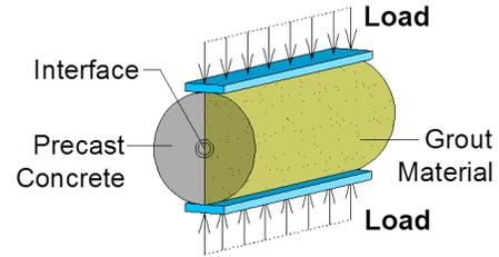
Figure 4. Slant-shear compression test for characterizing bond between precast concrete and field-cast connection grouts.
