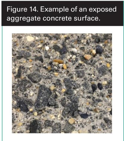
exposed aggregate surfaces leads to higher flexural bond strengths compared with other surface preparation methods applicable to precast concrete elements.
