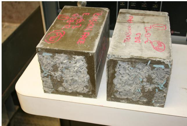
Figure 8. Typical failure modes exhibited in bond testing—failure location 3: failure in substrate.
