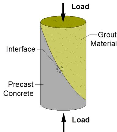
Figure 5. Direct tension pull-off test for characterizing bond between precast concrete and field-cast connection grouts.
