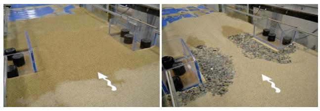
Figure 71. Photos. Comparison of run 6 as-built riprap installation (left) and at equilibrium scour (right).
