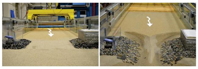
Figure 67. Photos. Comparison of run 4 as-built riprap installation (left) and at equilibrium scour (right).
