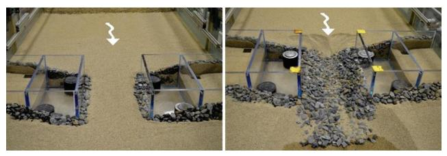
Figure 75. Photos. Comparison of run 9 as-built riprap installation (left) and at equilibrium scour (right).
