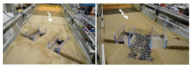
Figure 77. Photos. Comparison of run 11 as-built riprap installation (left) and at equilibrium scour (right).
