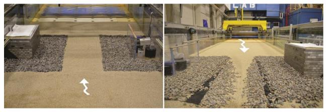
Figure 61. Photos. Comparison of run 1 as-built riprap installation (left) and at equilibrium scour (right).
