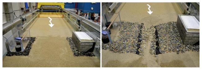
Figure 63. Photos. Comparison of run 2 as-built riprap installation (left) and at equilibrium scour (right).
