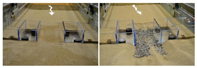
Figure 73. Photos. Comparison of run 8 as-built riprap installation (left) and at equilibrium scour (right).
