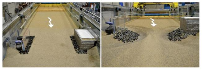
Figure 65. Photos. Comparison of run 3 as-built riprap installation (left) and at equilibrium scour (right).
