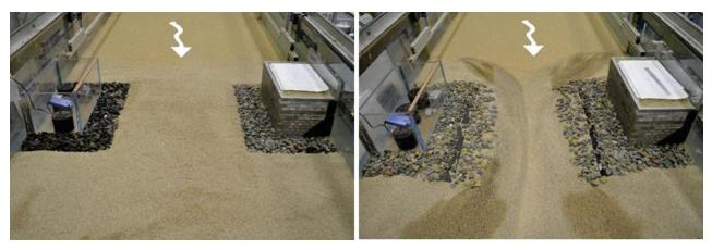
Figure 69. Photos. Comparison of run 5 as-built riprap installation (left) and at equilibrium scour (right).
