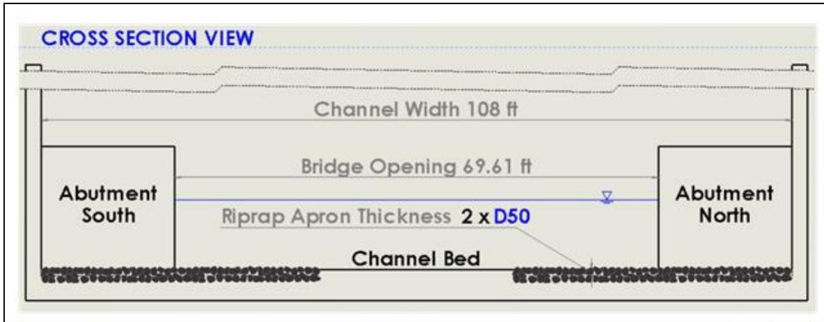
**Figure 14. Sketch. Cross-section view of the prototype domain.**
