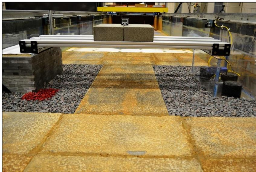
**Figure 8. Photo. Riprap apron installation for testing.**
