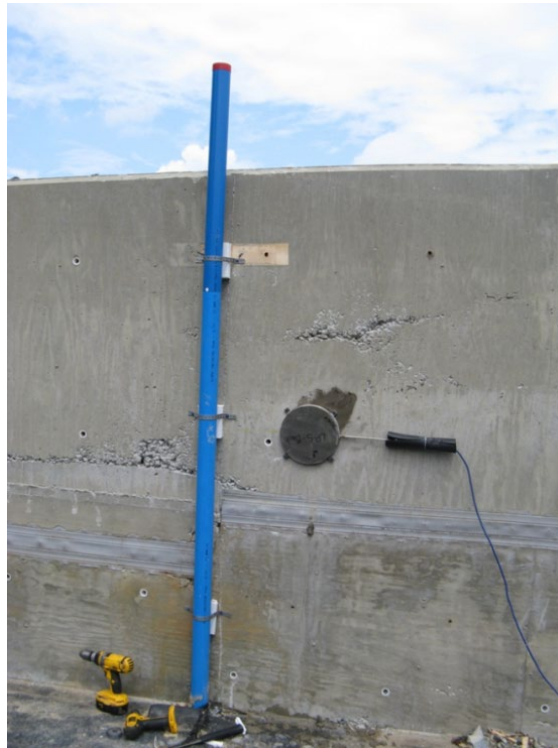
Figure 44. Photo. Close-up view of an IPI used to measure thermally induced movement.
