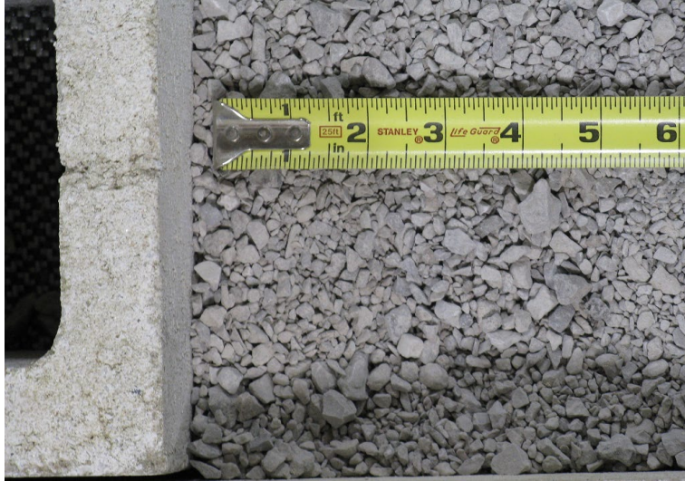
Figure 4. Photo. Sample open-graded aggregate.
