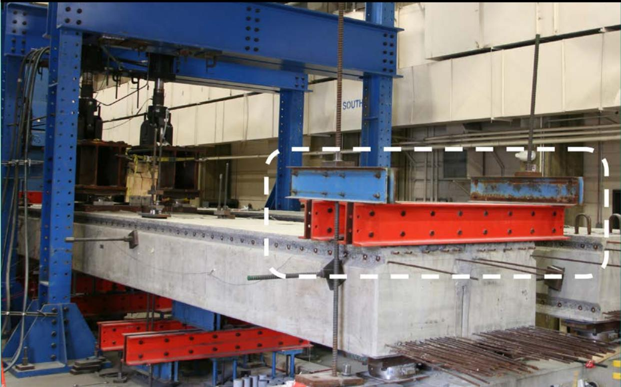
Figure 5. Intermediate support on one beam used in the fully stiffened case.
