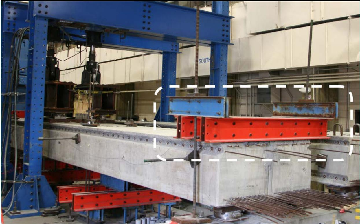
Figure 5. Intermediate support on one beam used in the fully stiffened case.
