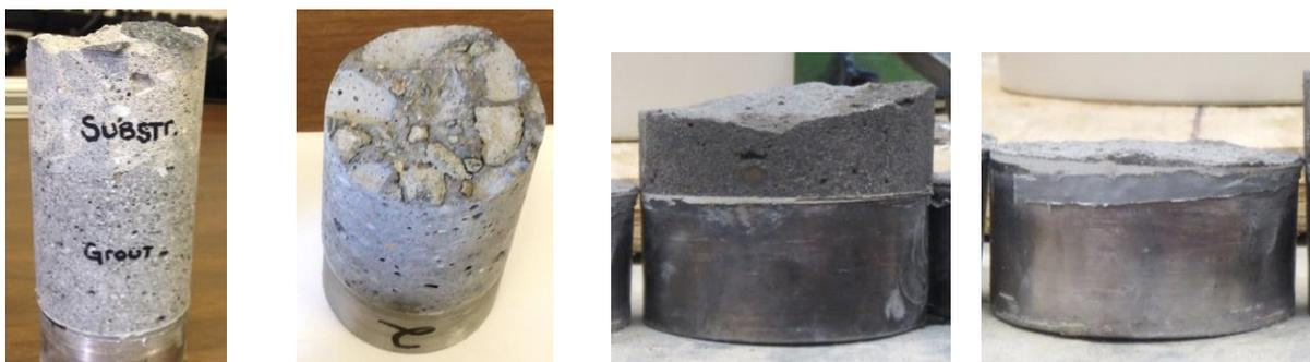
A. Mode 1: Substrate failure.
