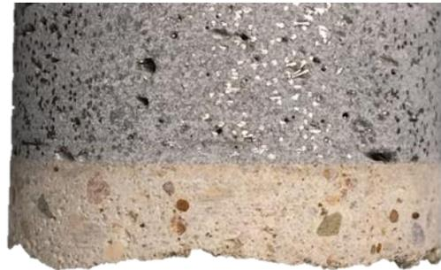
C. UHPC-concrete interface of G3-13 specimen after testing.
