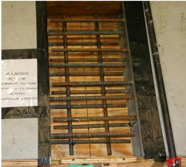
A. Example of transverse reinforcement for straight lap spliced bars
