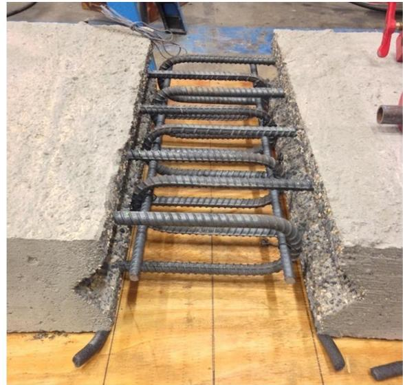
B. Example of transverse reinforcement for lap spliced U-bars
