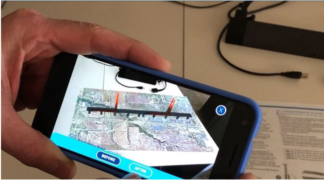
Figure 4. Photo. 3D model view overlaid on live video through a mobile device.
