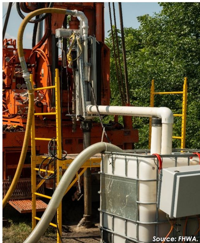
The ISTD equipment assembled in front of the drill rig.
