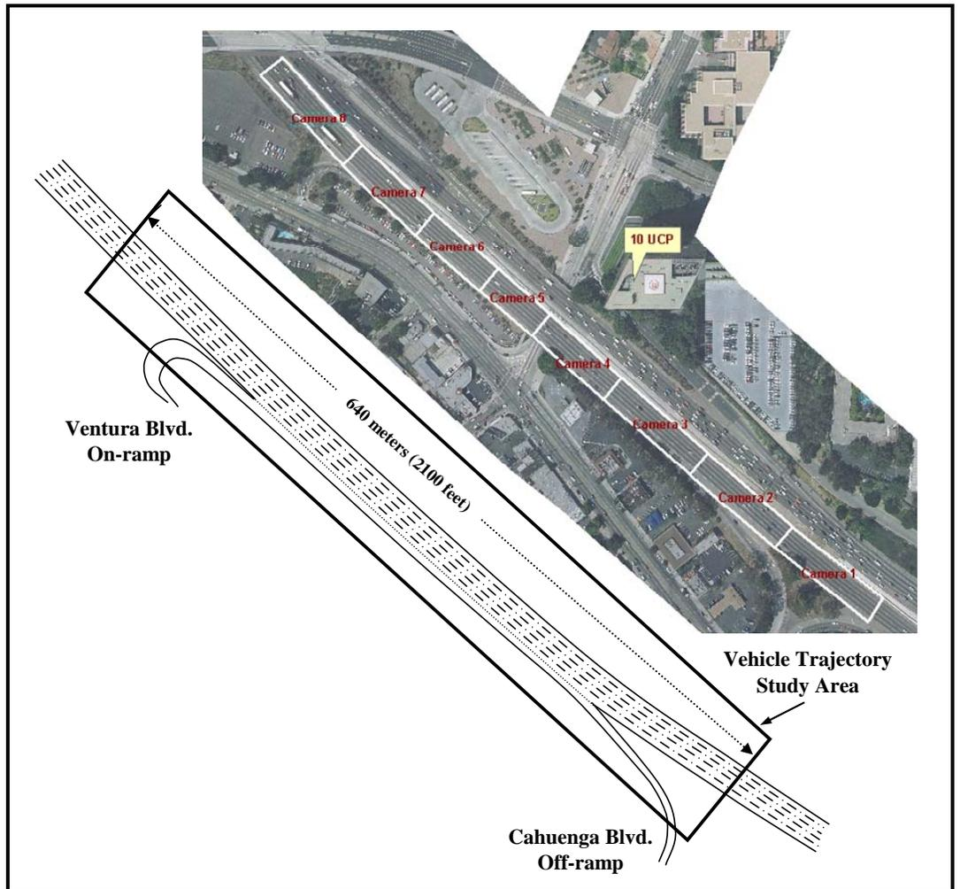
**Figure 1.** The aerial photograph above shows the extent of the US 101 study area in relation to the building from which the digital video cameras were mounted and the coverage area for each of the eight cameras. The schematic drawing on the bottom shows the number of lanes and location of the on-ramp at Ventura Boulevard and the off-ramp at Cahuenga Boulevard within the US 101 study area.
