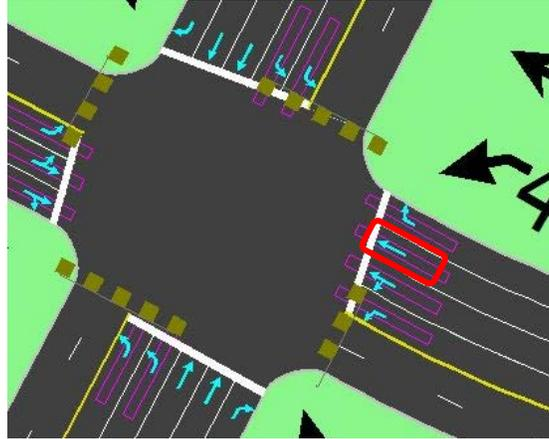
**Figure 41. Illustration. Lane assignment before DLG for case study 1.**
