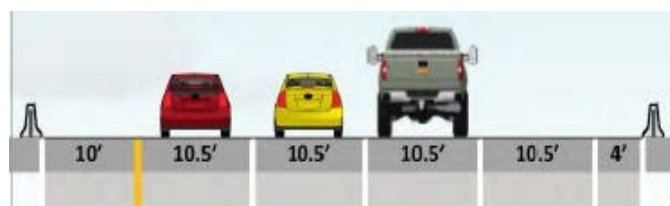
Source: FHWA Figure 6. Lane narrowing to add a new lane.
