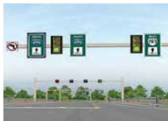
Figure 3(a). On-peak upstream signalized intersection recommendations (DRLT).
