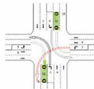
Figure 2. Signalized intersection with CLT treatment creating an additional dynamic LT bay using OTL during minor street green phase. 1
