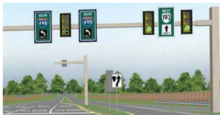
Figure 5. On-peak downstream gantry recommendations (DRLT); during off-peak, leftmost changeable message sign will display a white-on-black "THIS LANE CLOSED" message.
