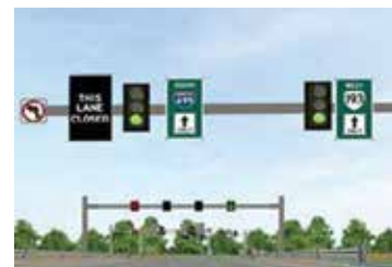
Figure 3(b). Off-peak upstream signalized intersection recommendations (DRLT).
