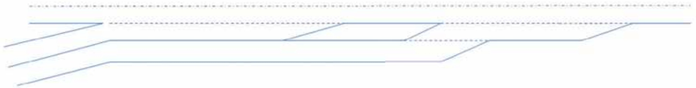
Figure 1. Acceleration lane with two merge points. (Source: FHWA)
