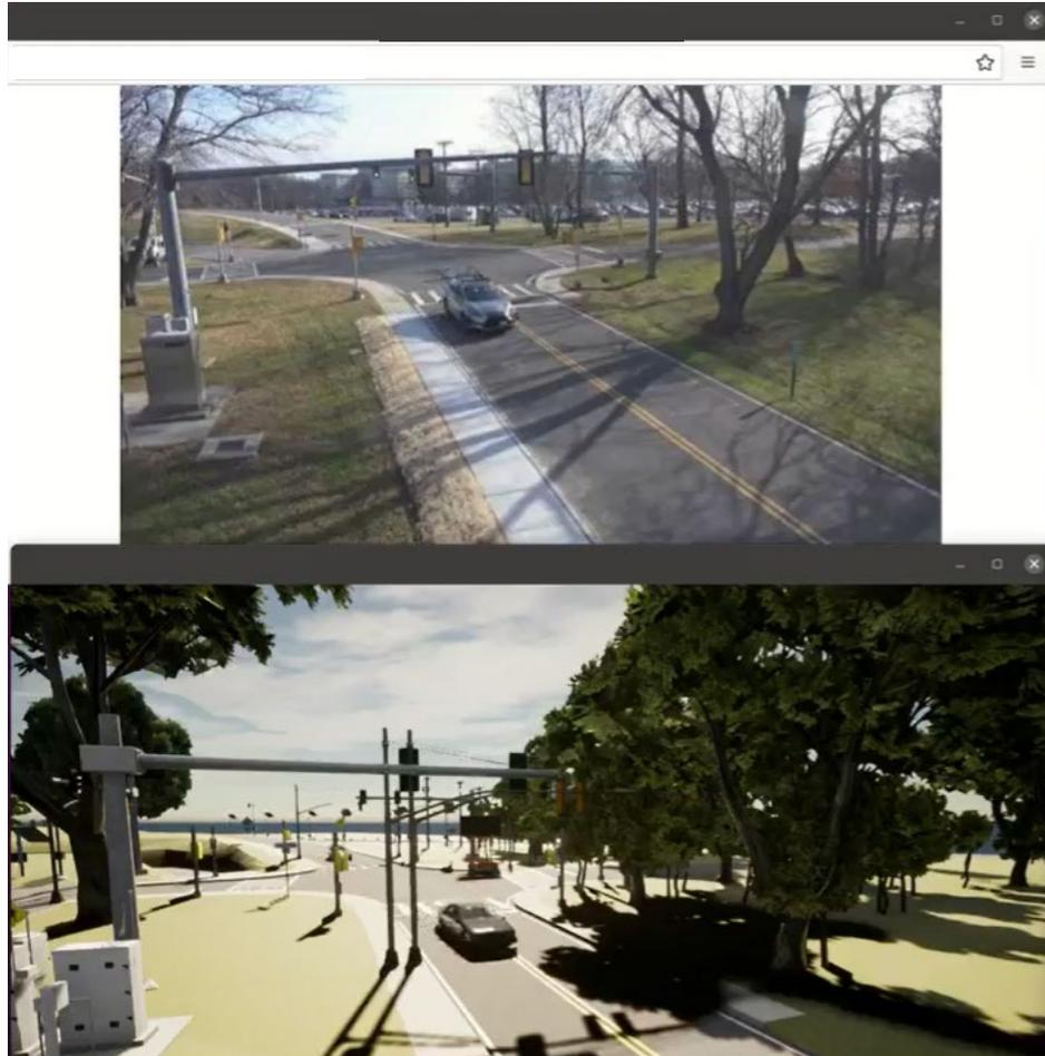
VOICES is demonstrated in this image, which depicts a live vehicle driving along a roadway while its virtual counterpart is displayed in a CARLA simulation running in a computer. This image highlights the possibility of experimenting with live and virtual interactions using a common set of adapters and interfaces.
