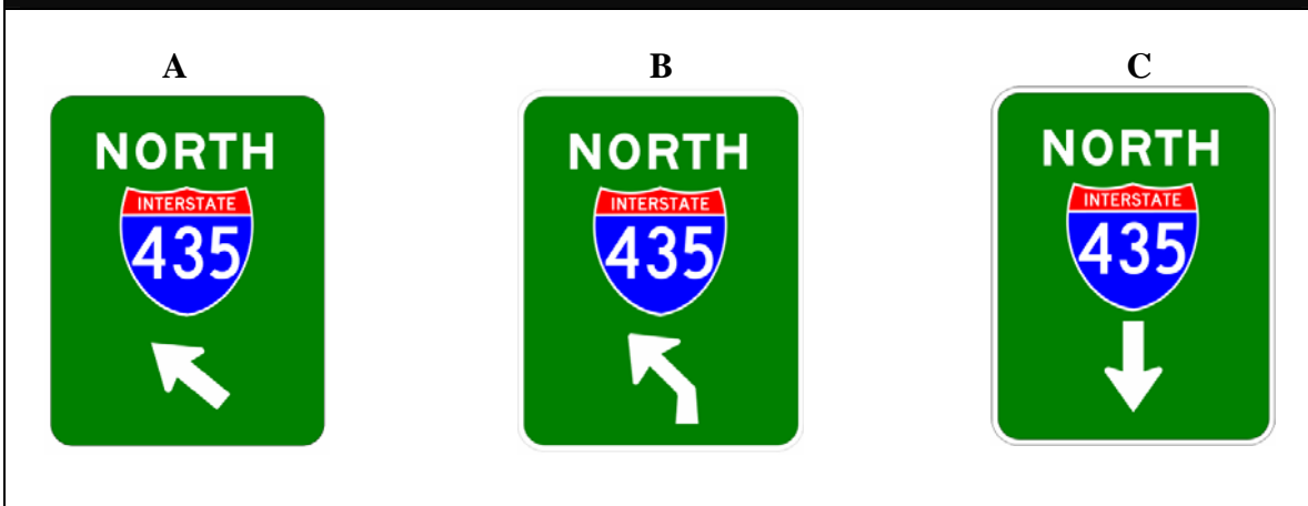
Figure 9. The figure shows three types of overhead navigation signs. The sign labeled A was used above the underpass, although B or C would have been more appropriate for a turn beyond the underpass.
