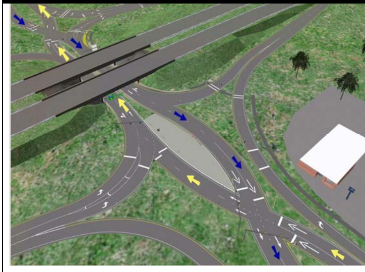
Figure 1. Aerial view of a simulated DDI. Yellow and blue arrows indicate the direction of travel on the arterials.
