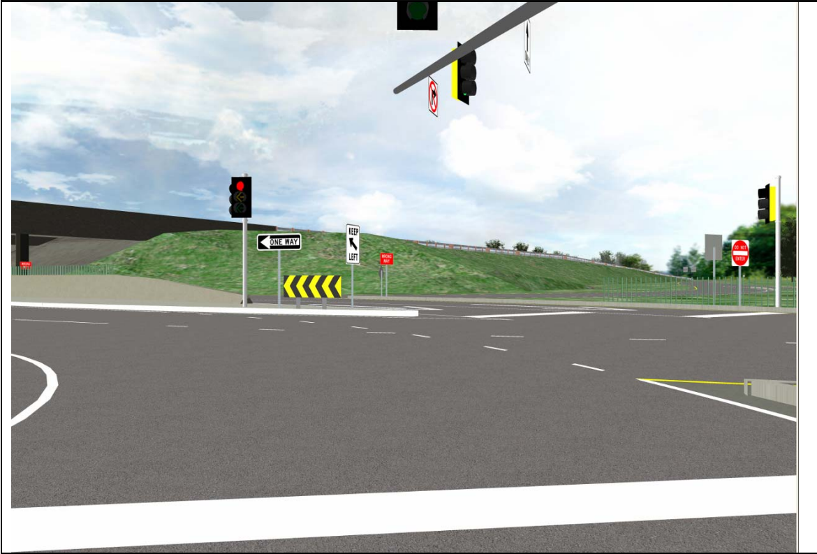
Figure 6. The crossover on the eastern node of the interchange where drivers on the northbound offramp could see a path to the opposing eastbound lanes.
