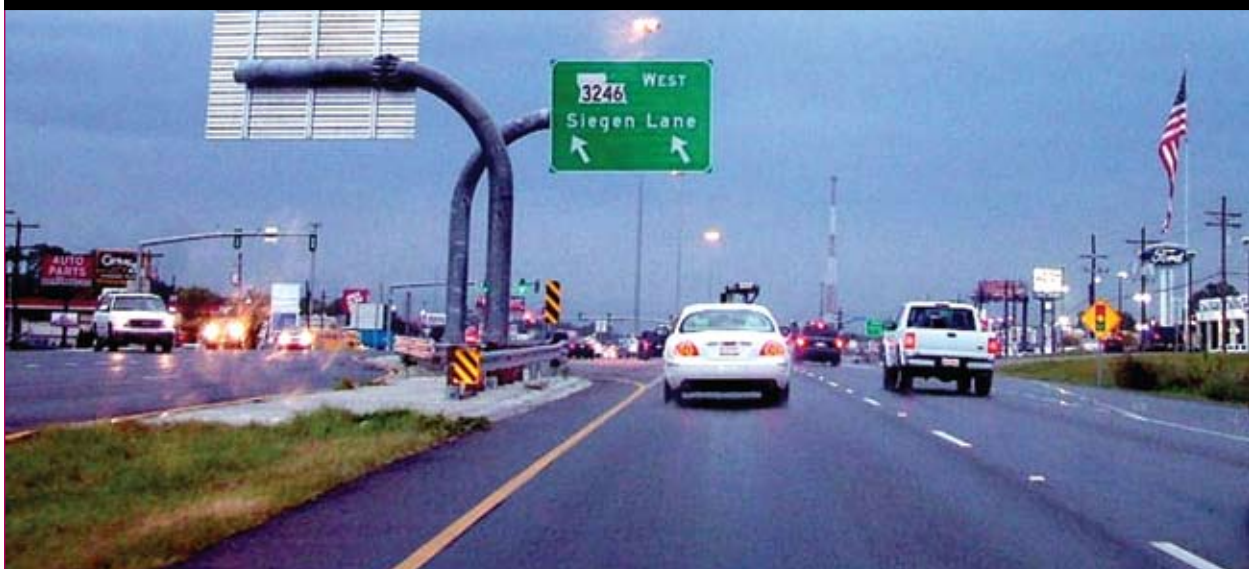
Figure 4. Overhead sign for a left-turn crossover at the Baton Rouge DLT.
