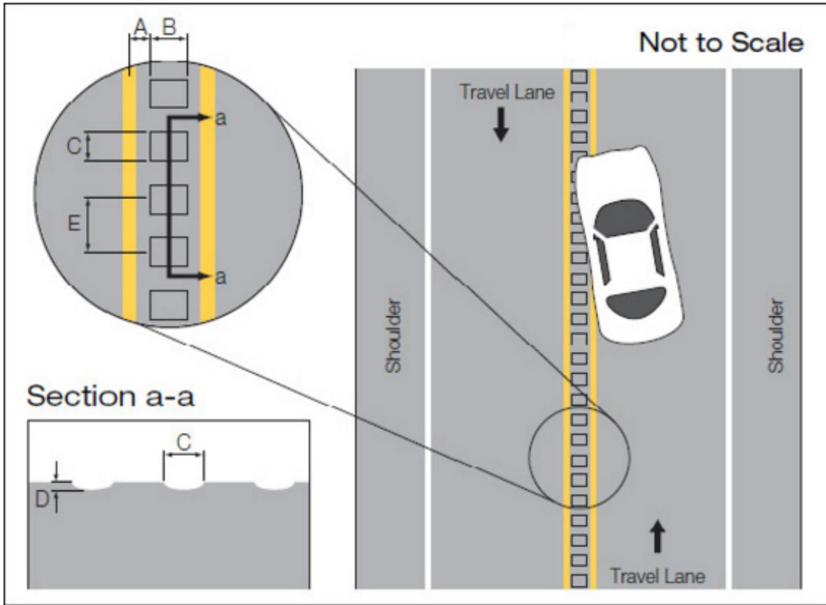
**Figure 8. Illustration. CLRS dimensions.<sup>(7)</sup>**
