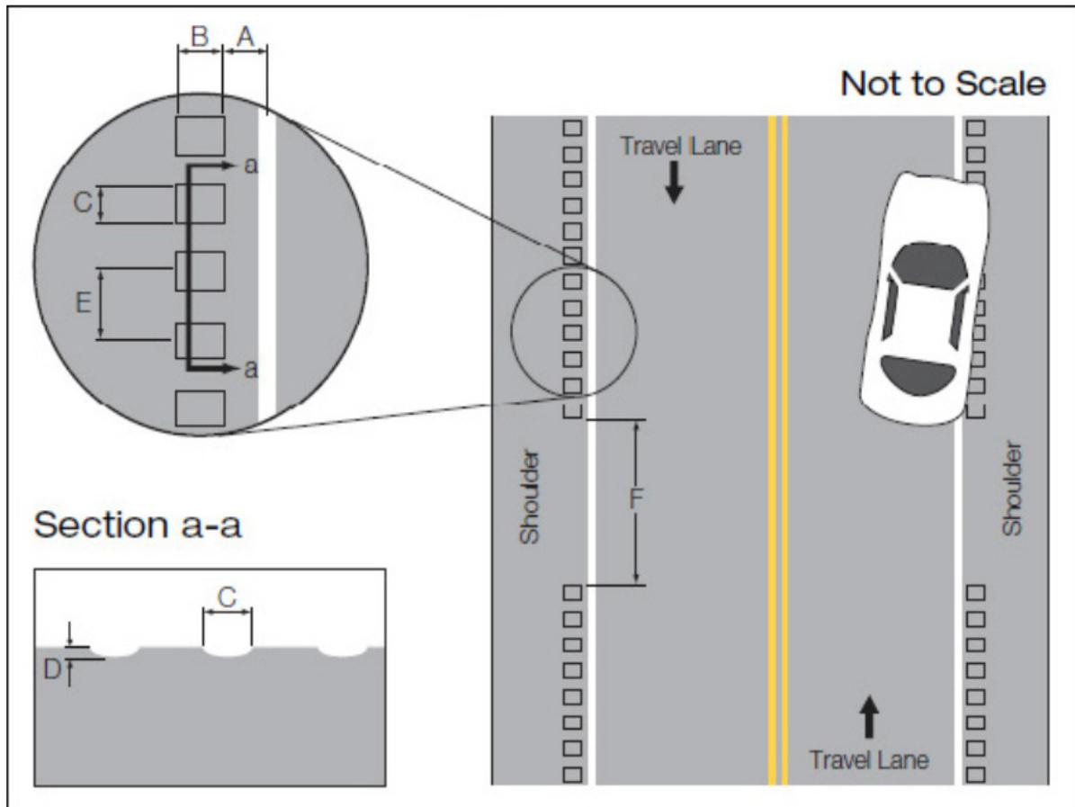
Figure 4. Illustration. Overview of rumble strip dimensions.<sup>(7)</sup>
