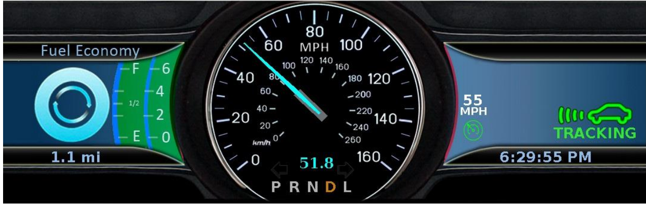
Figure 5. Photo. Instrument cluster with display of tracking status.
