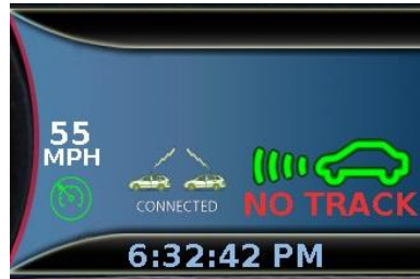
Figure 5. Photo. Instrument cluster with display of tracking status.
