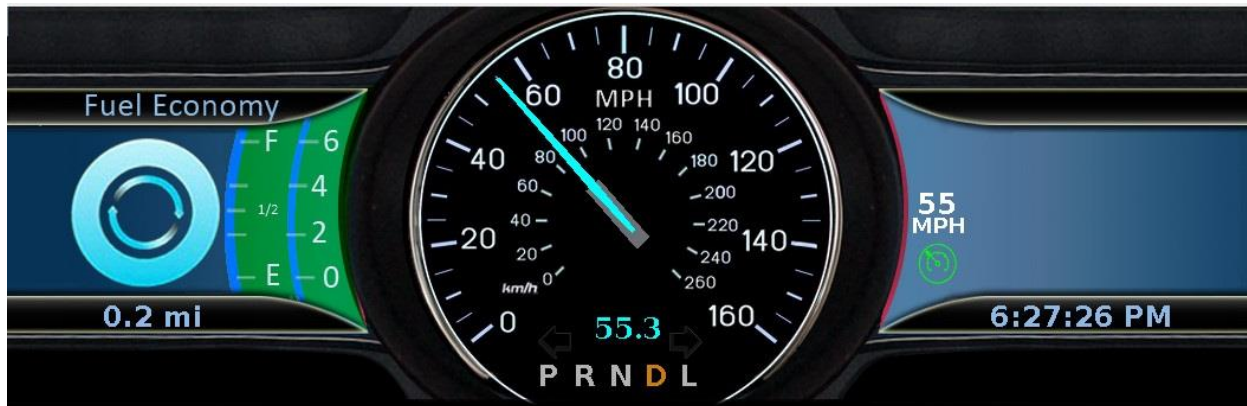
Figure 4. Photo. Instrument cluster with display showing cruise control on.
