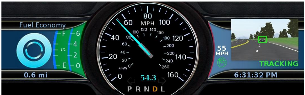
Figure 7. Photo. ACC instrument cluster with video of the road ahead.
