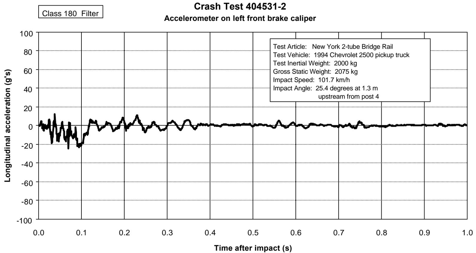
Figure 25. Vehicle longitudinal accelerometer trace for test 404531-2 (accelerometer located on left front brake caliper).
