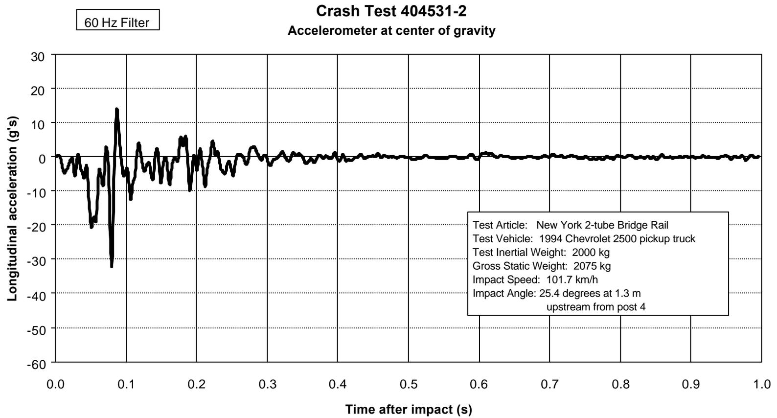
Figure 17. Vehicle longitudinal accelerometer trace for test 404531-2 (accelerometer located at center of gravity).
