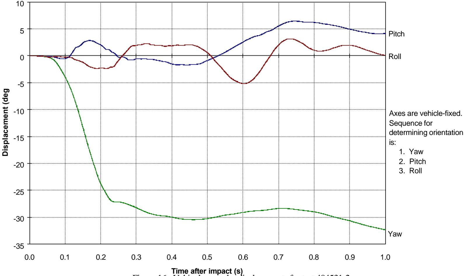
Figure 16. Vehicular angular displacements for test 404531-2.
