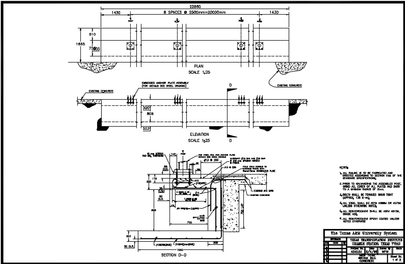
Figure 1. Details of the New York Curbless Two-Rail Bridge Railing for test 404531-1.
