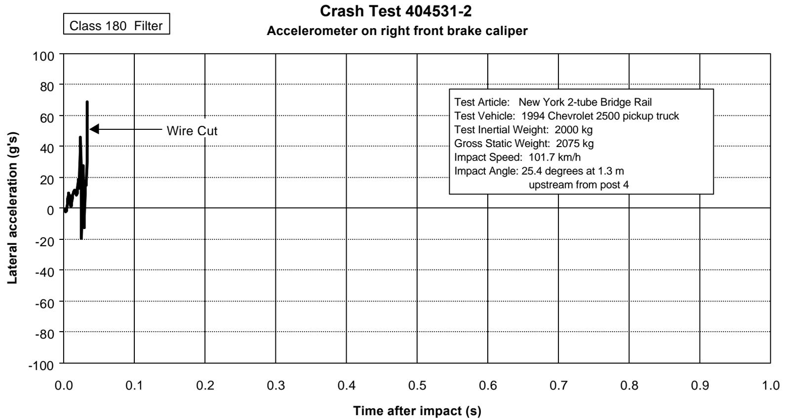
Figure 24. Vehicle lateral accelerometer trace for test 404531-2 (accelerometer located on right front brake caliper).
