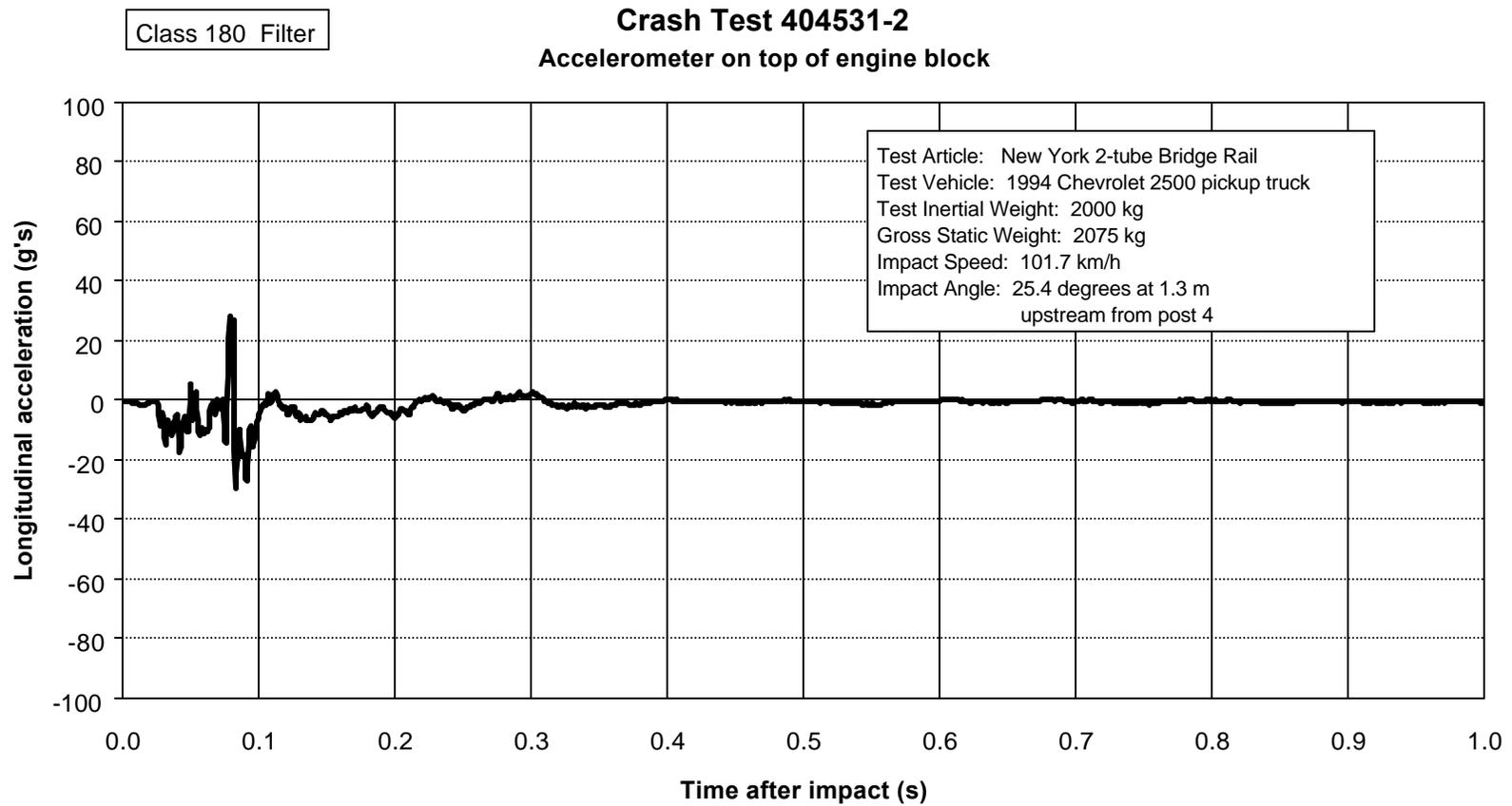
Figure 26. Vehicle longitudinal accelerometer trace for test 404531-2 (accelerometer located on top of engine block).
