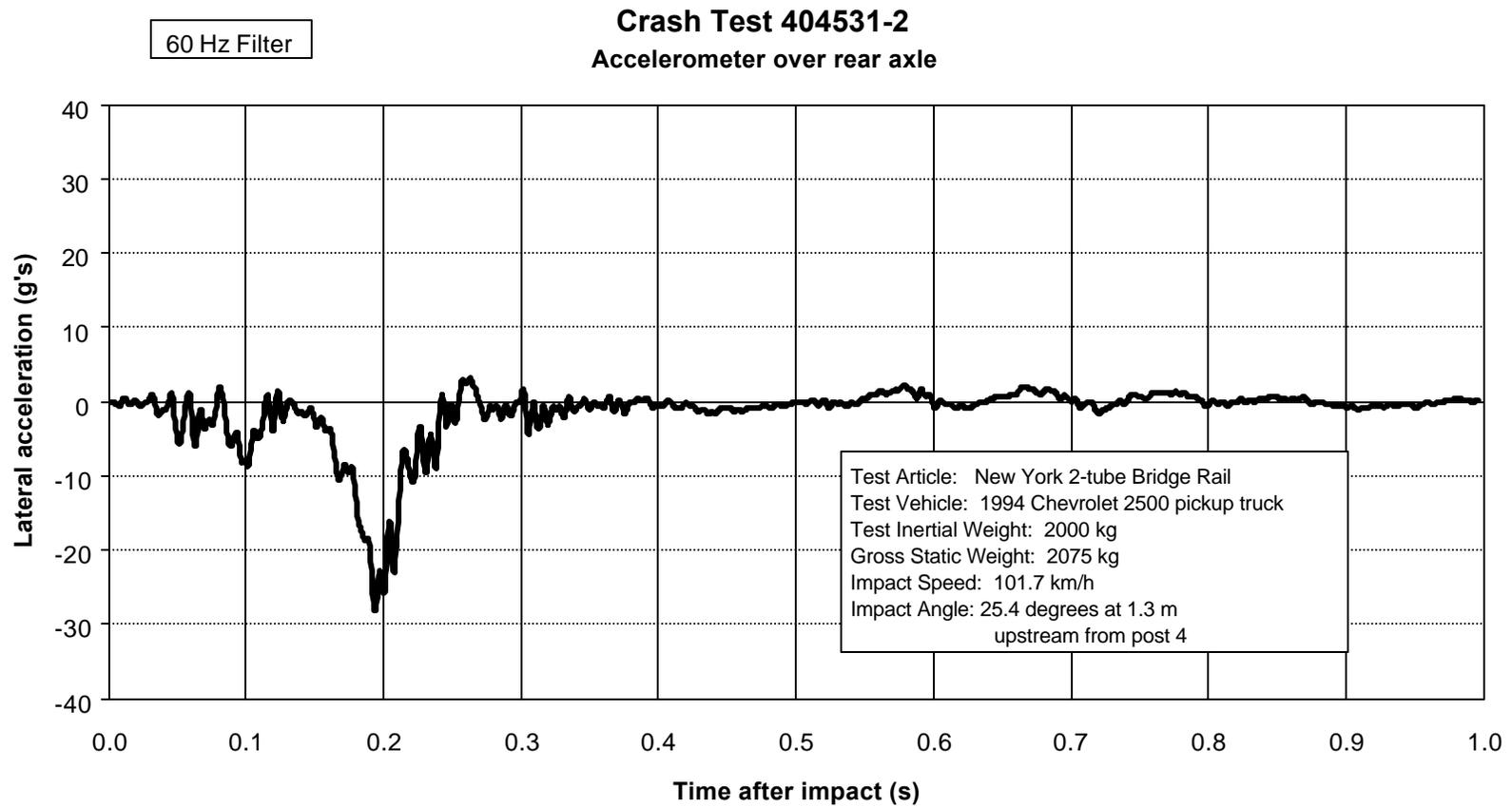
Figure 21. Vehicle lateral accelerometer trace for test 404531-2 (accelerometer located over rear axle).
