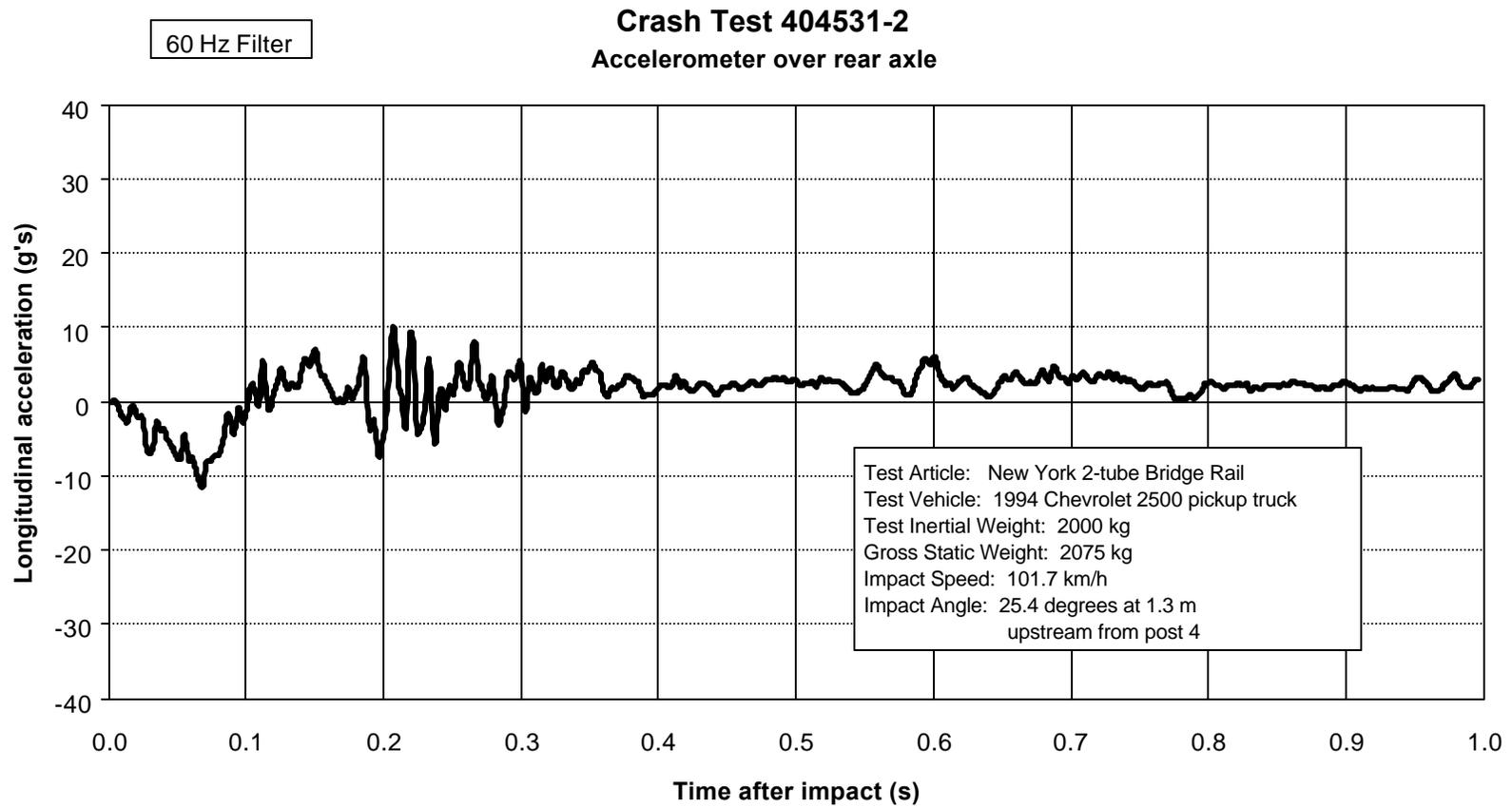
Figure 20. Vehicle longitudinal accelerometer trace for test 404531-2 (accelerometer located over rear axle).
