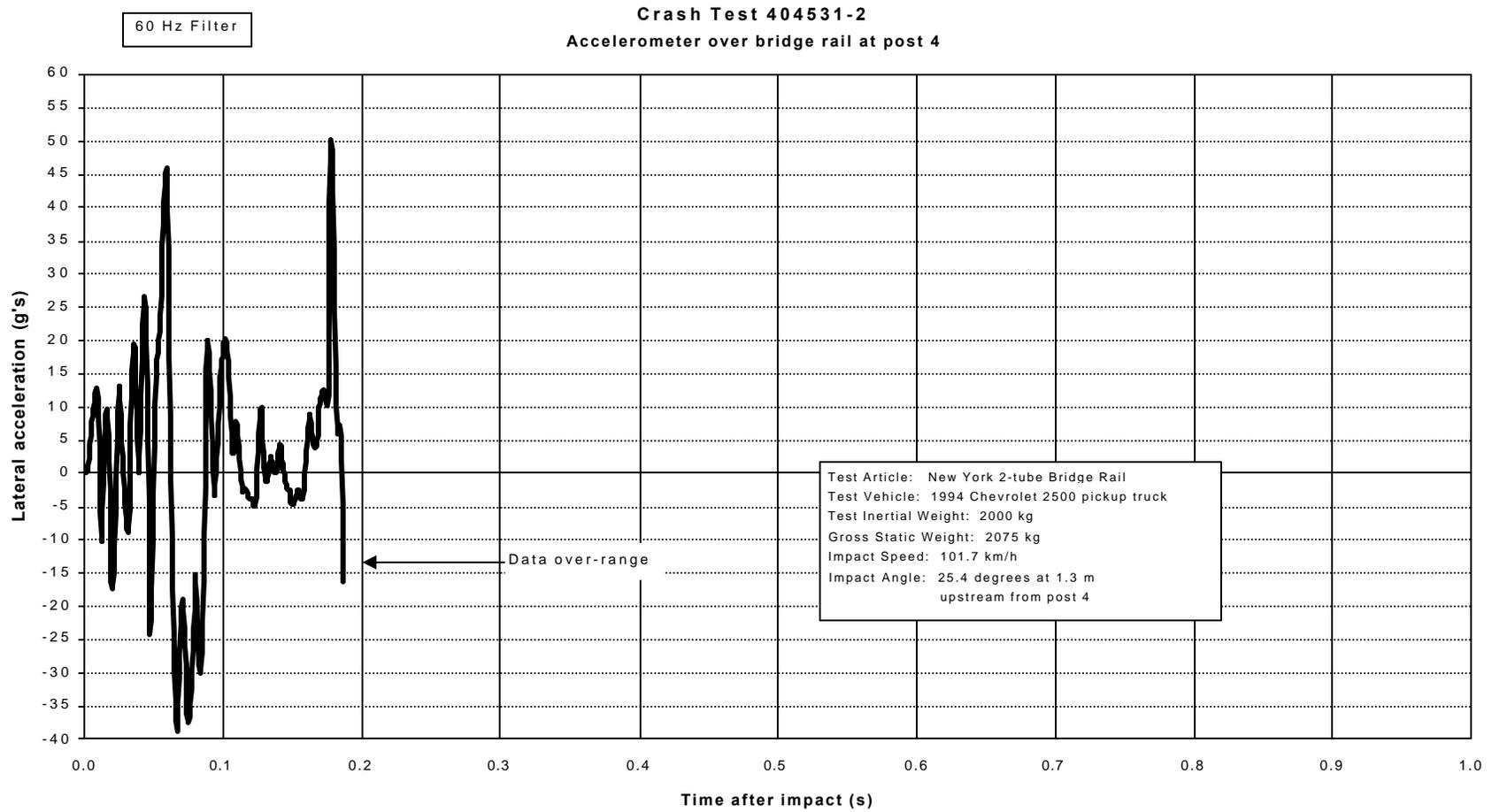
Figure 29. Bridge rail lateral accelerometer trace for test 404531-2 (accelerometer located over bridge rail at post 4).
