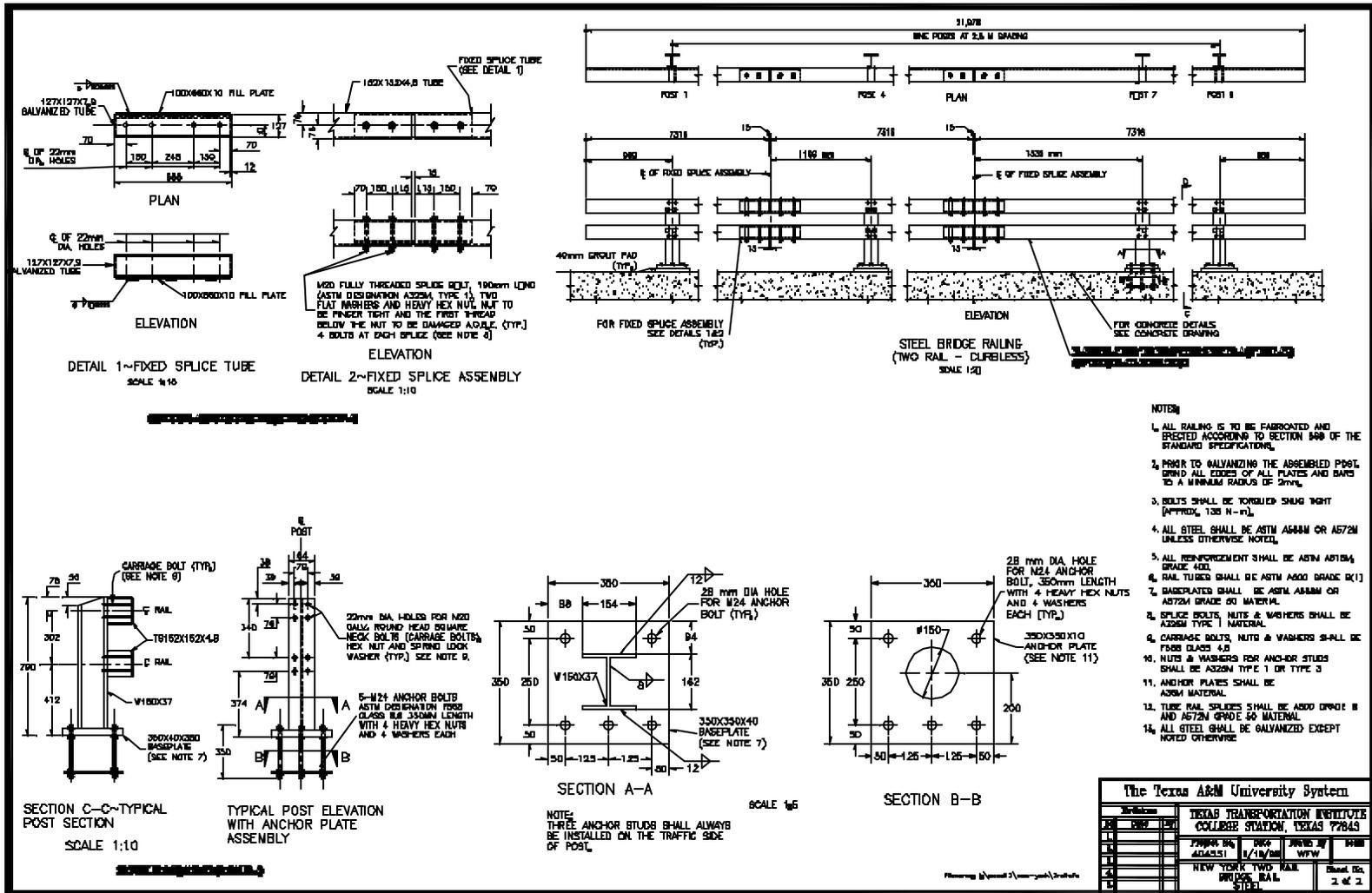
Figure 2. Layout of test installation.
