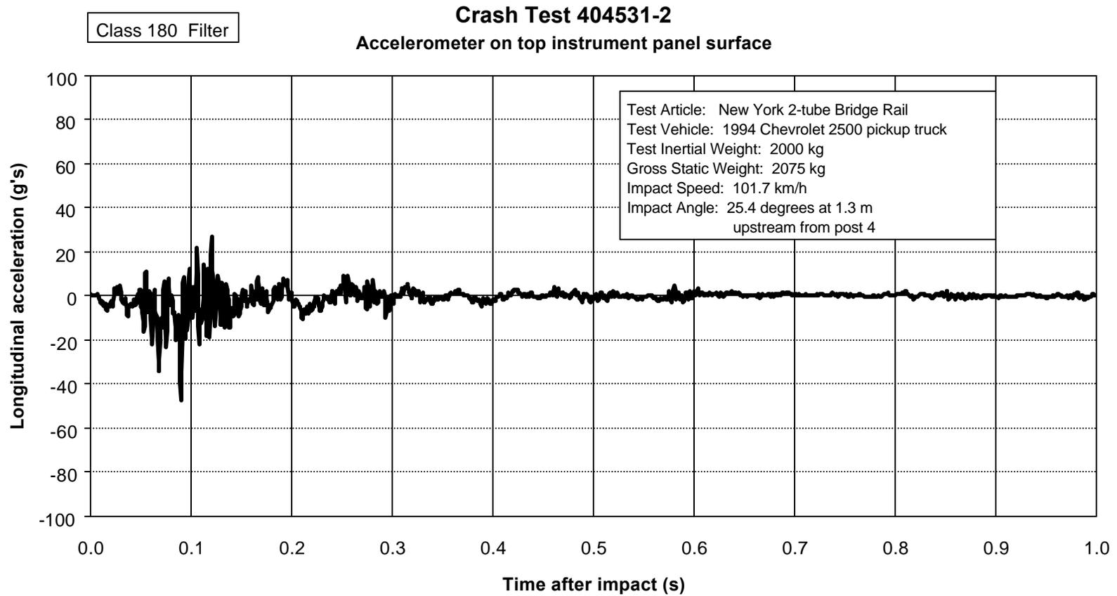
Figure 23. Vehicle longitudinal accelerometer trace for test 404531-2 (accelerometer located on top surface of instrument panel).
