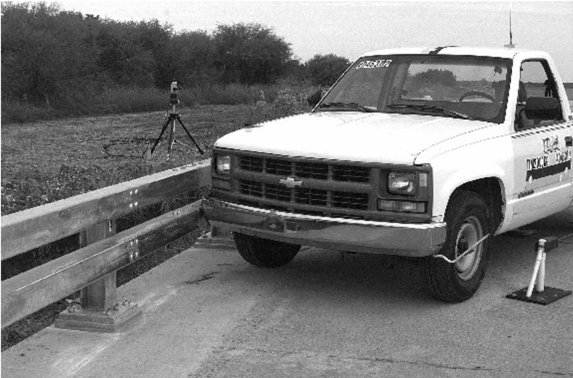
Figure 5. Vehicle/installation geometrics for test 404531-2.
