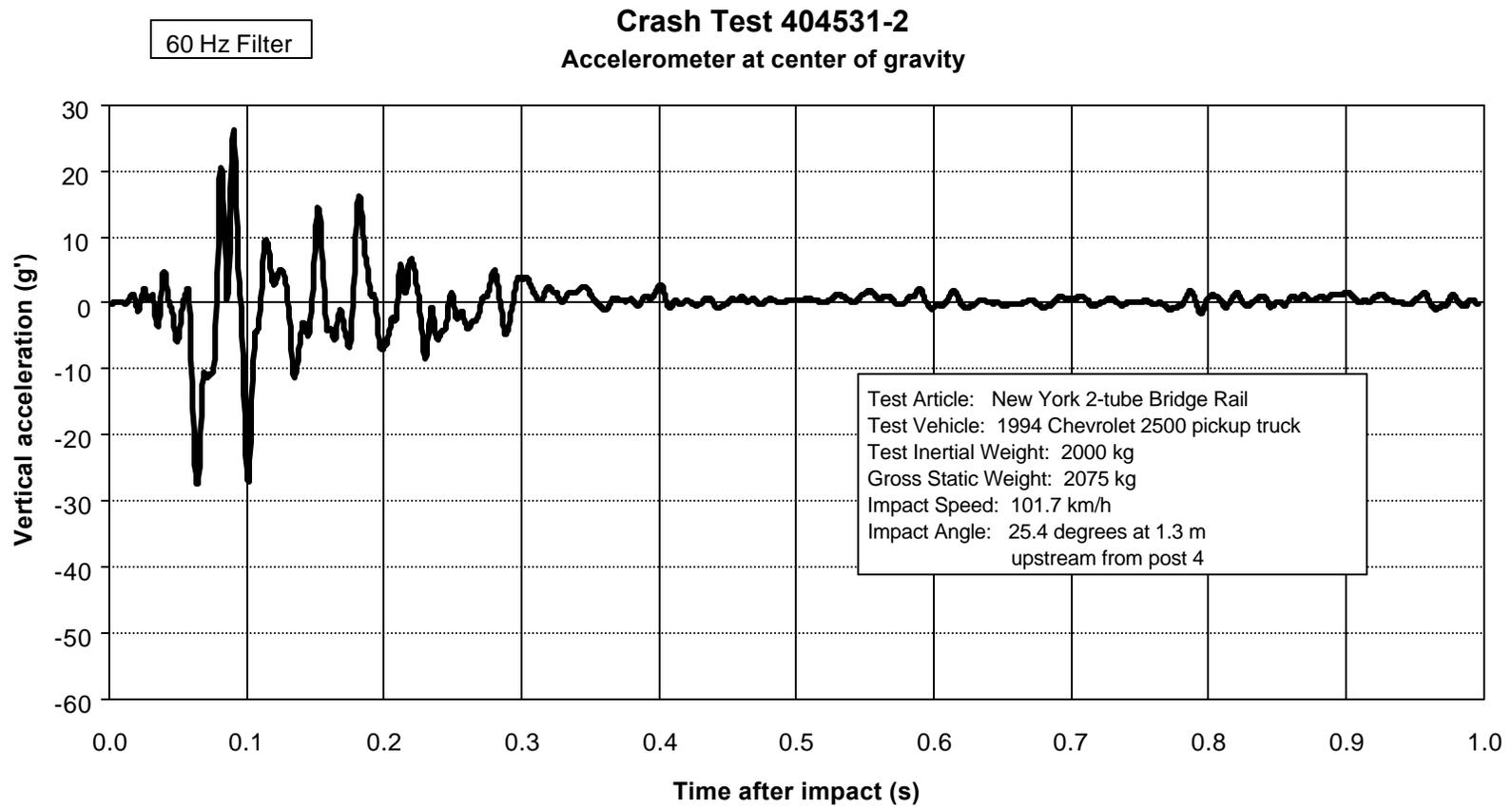
Figure 19. Vehicle vertical accelerometer trace for test 404531-2 (accelerometer located at center of gravity).
