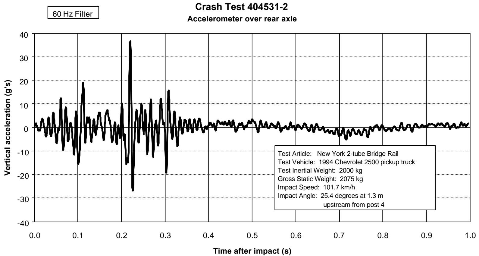
Figure 22. Vehicle vertical accelerometer trace for test 404531-2 (accelerometer located over rear axle).
