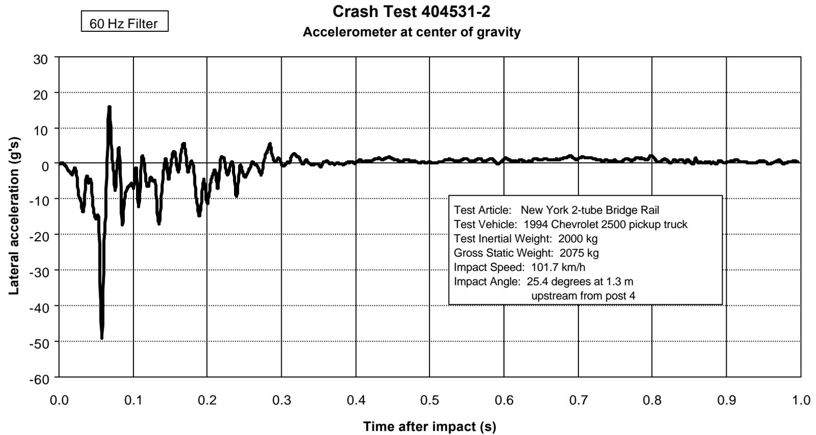
Figure 18. Vehicle lateral accelerometer trace for test 404531-2 (accelerometer located at center of gravity).
