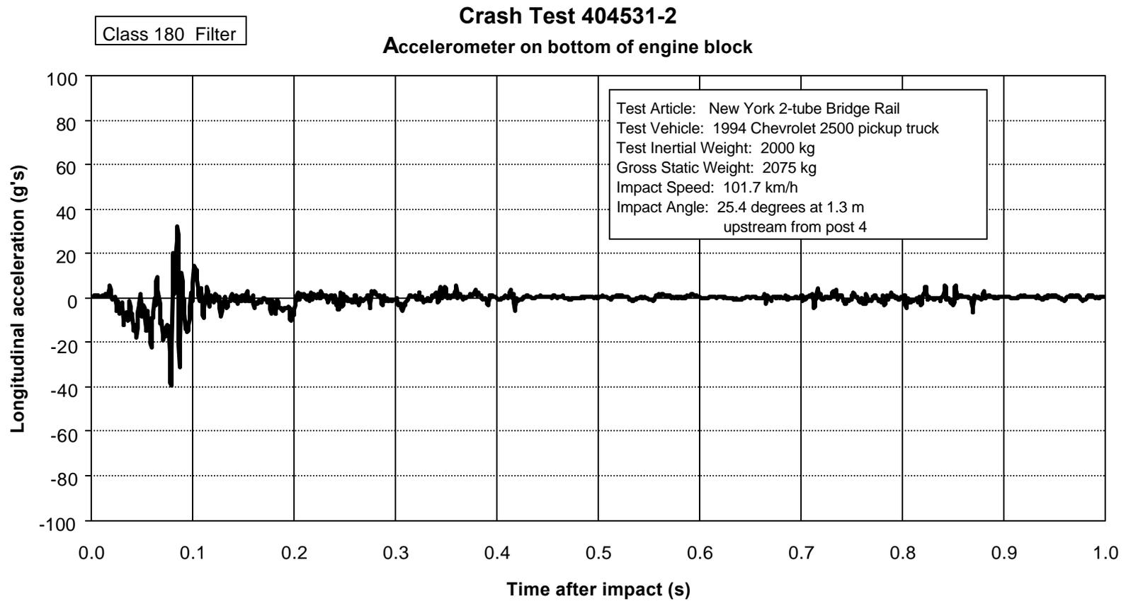
Figure 27. Vehicle longitudinal accelerometer trace for test 404531-2 (accelerometer located on bottom of engine block).
