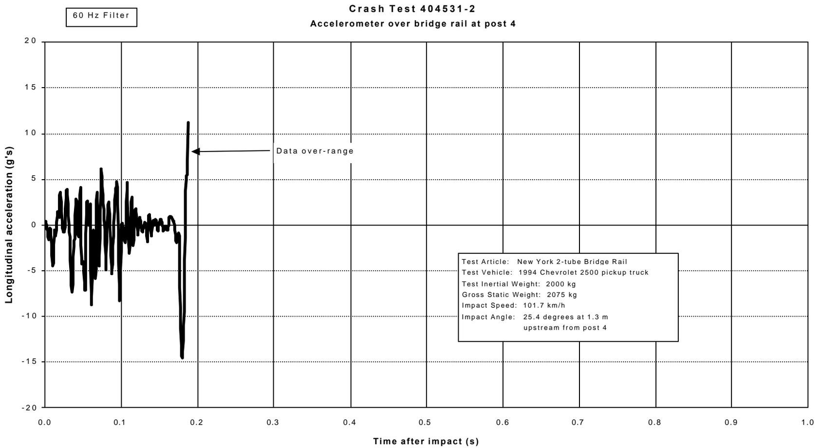
Figure 28. Bridge rail longitudinal accelerometer trace for test 404531-2 (accelerometer located over bridge rail at post 4).
