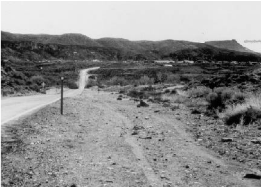
Figure 9. Typical Roadway with Roadside Hazard Rating Equal to 2.
