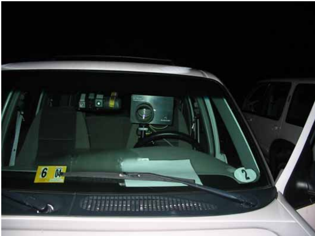
Figure 25. Photo. CCD photometer in experimental vehicle, front view.
