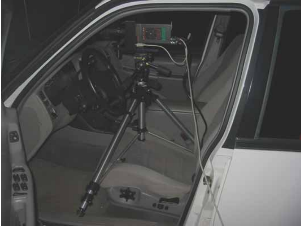
Figure 24. Photo. CCD photometer in experimental vehicle, side view.
