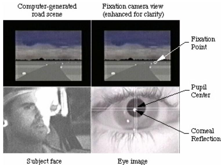
Note: The image of the subject's face suggests a blinding light was illuminating it. In fact, the source was infrared, detectable by a video camera but barely detectable by a human eye.
