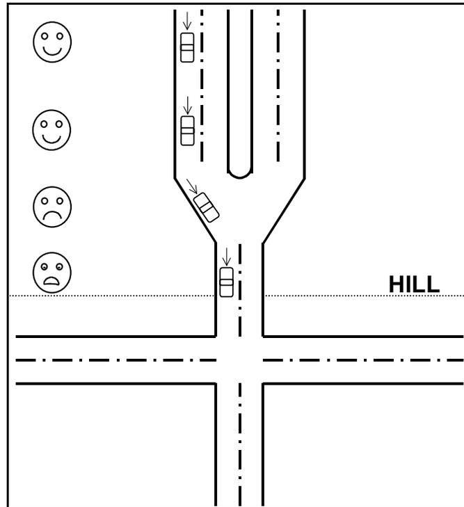
**Figure 1. Example of Inconsistent Design.**<sup>(31)</sup>
