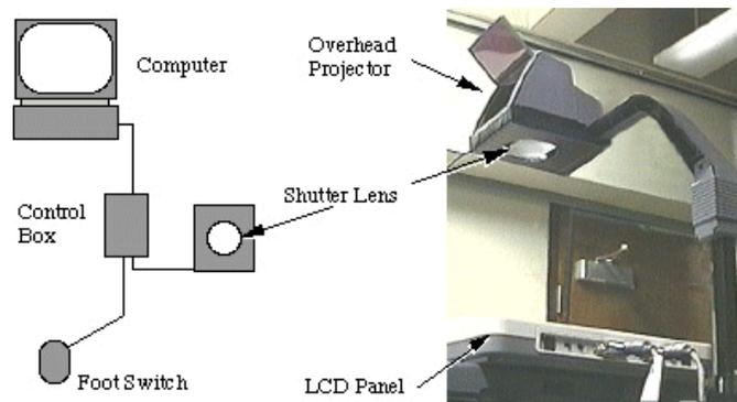
**Figure 34. Occlusion Shutter as Installed on the Overhead Projector for the Road Scene.**
