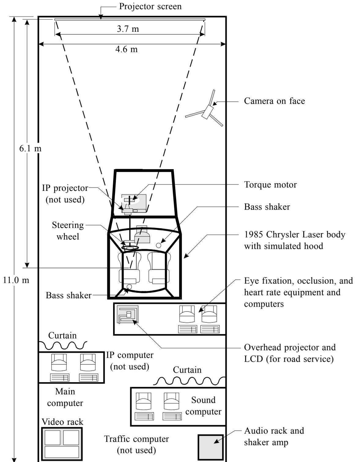
Figure 32. Plan View of the Driving Simulator Facility.
