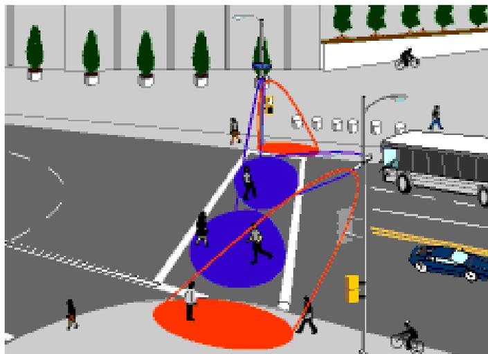
**Figure 10-14. Example of a microwave detector system.**
