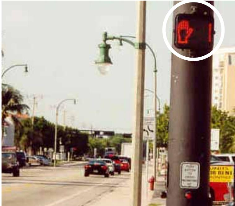
**Figure 10-12. Photo. Example of countdown pedestrian signal in Lauderdale-By-The-Sea, FL.**
