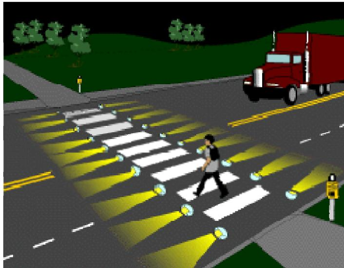
**Figure 10-10. Illustration. Example of in-roadway warning lights.**
