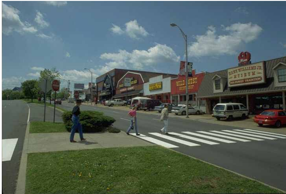
Figure 7-6. Photo. Medians and crosswalks should be placed at destination locations such as this shopping center.
