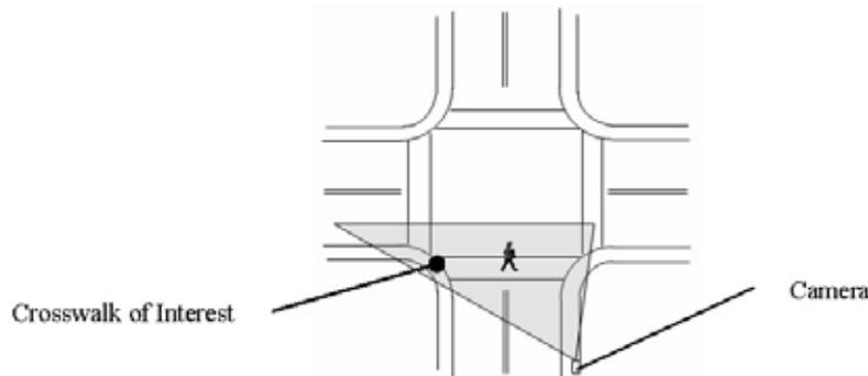
**Figure 2. Video camera position for pedestrian data collection.**
