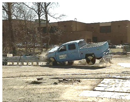
A pickup truck crashes into a bridge-end barrier at the FOIL crash test facility in McLean, VA.
