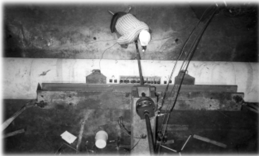
The shaft was supported on each end and loaded along the middle section. Deformation was monitored and cracks were mapped during the course of the experiments.
