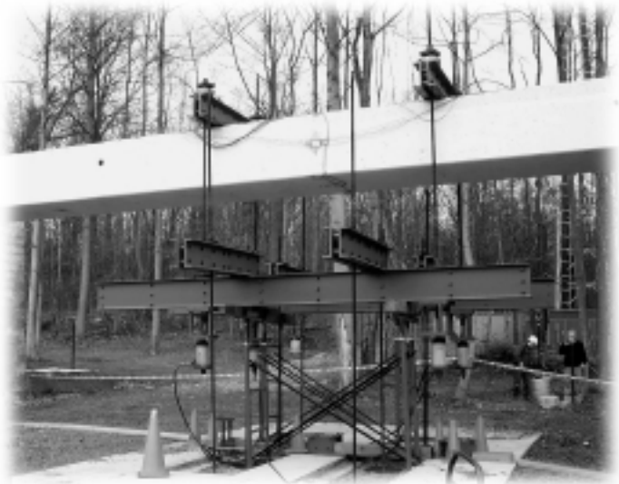
Testing of a box girder at the Turner-Fairbank Highway Research Center (TFHRC).
