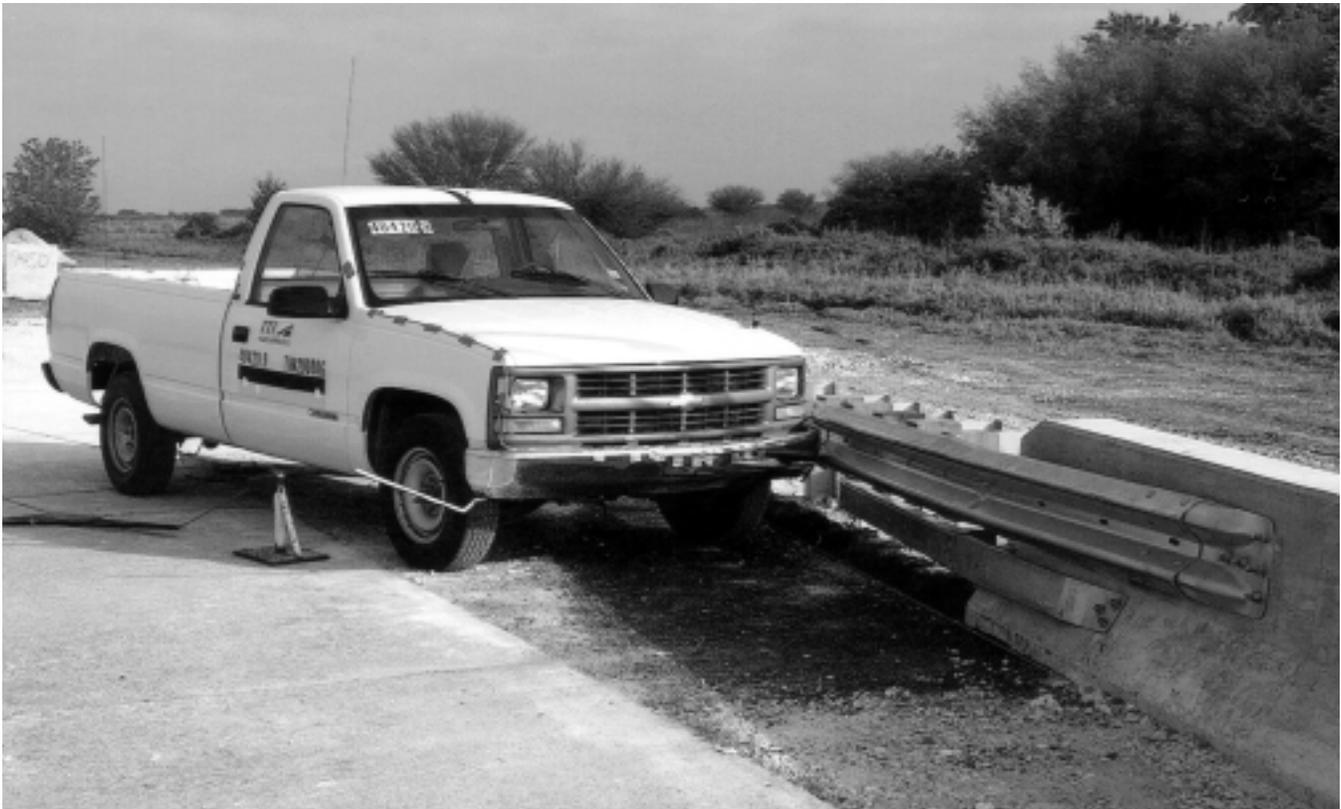
A test of the Connecticut transition successfully redirected this pickup truck with moderate damage to the transition.
