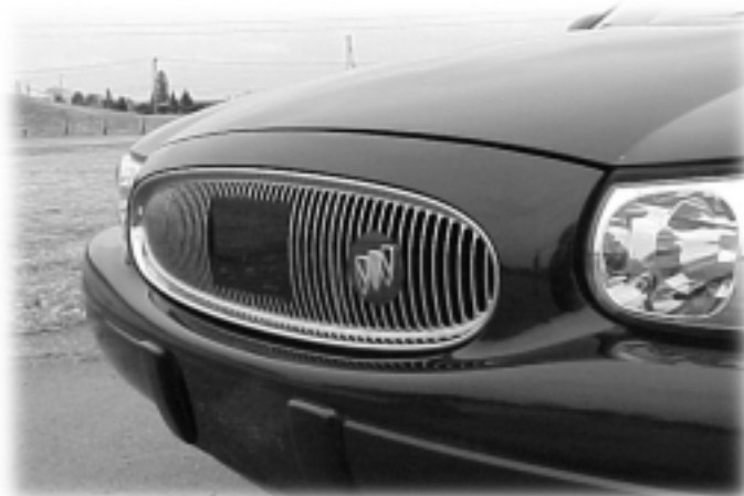
Radar mounted on the grill of an automobile helps prevent collisions.
