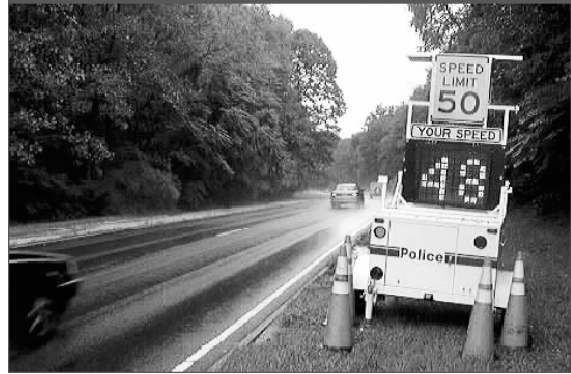
Speed Feedback display encourages speeding drivers to comply to posted limit
