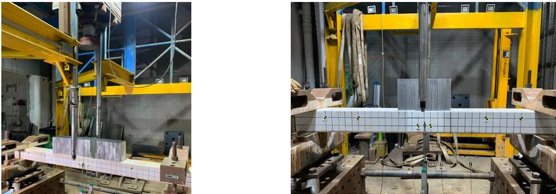
(a) Test setup of the steel beam with honeycombs. (b) Test setup showing the displacement sensor.
