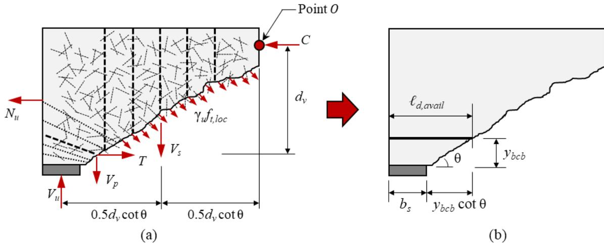
**Figure 41. Illustration. (a) Assumed failure crack in resistance model development and (b) available development length for reinforcement at failure crack.**
