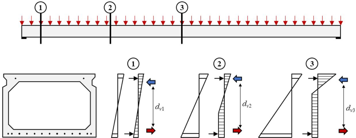
**Figure 40. Illustration. Changing strain and stress profile along length of beam and corresponding effective shear depth.**
