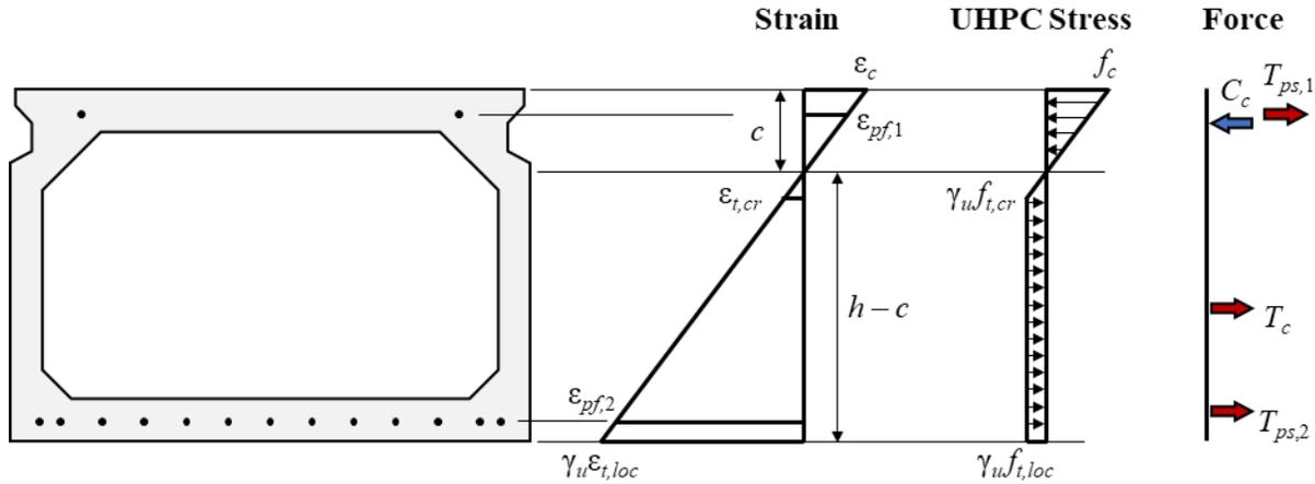
**Figure 39. Illustration. Strains, stresses, and forces at crack localization for Storyline Example 2.**
