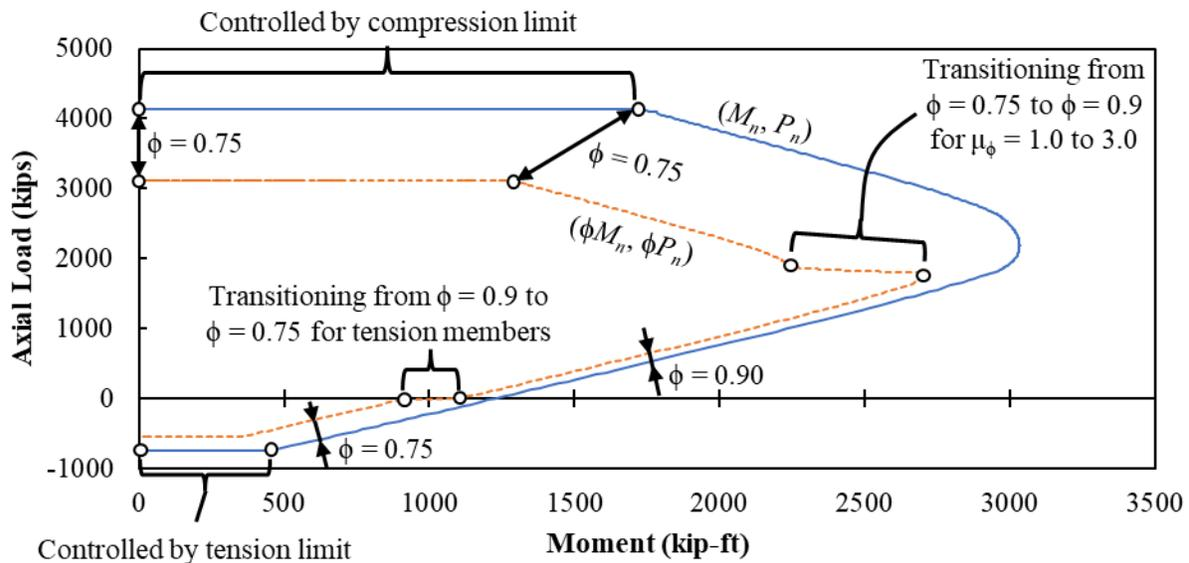
**Figure 26. Graph. Example of factored moment-axial load interaction diagram for Storyline Example #3.**
