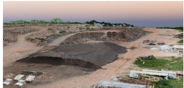
Figure 7: Image pulled from a Duit Construction video demonstrating using topographical imagery to assess material volumes in a recycle yard.
