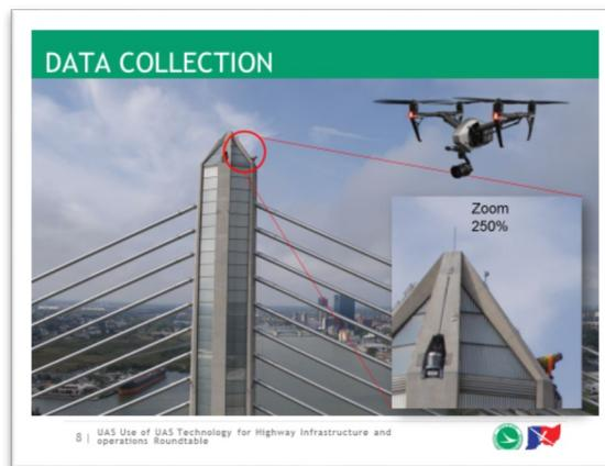
Figure 1: Ohio DOT image illustrating the zoom capabilities of its UAS equipment.
