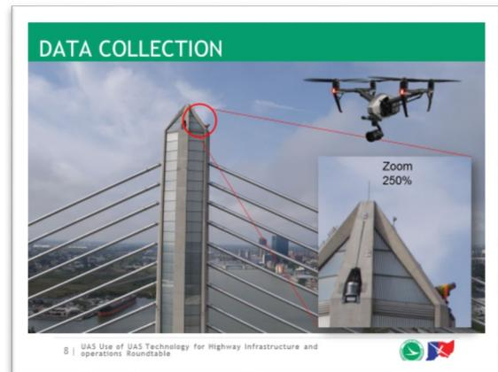
Figure 1: Ohio DOT image illustrating the zoom capabilities of its UAS equipment.
