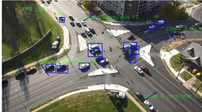
Figure 6: Image from Ohio DOT's UAS Demonstrating Traffic Counting Software.
