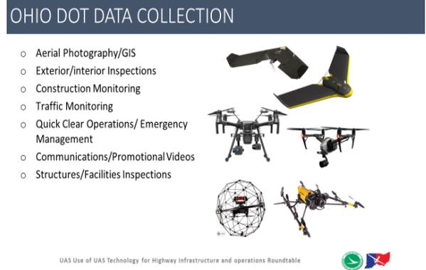
Figure 3: Types of UAS equipment employed at Ohio DOT for data collection operations.
