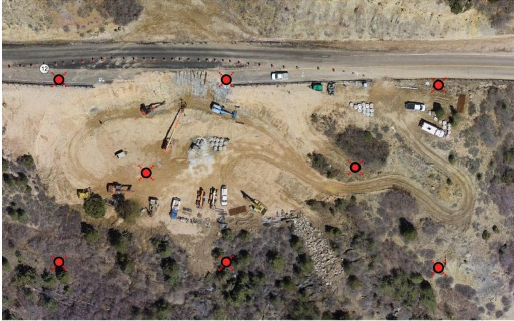
**Figure 14. UDOT GCP Layout on Construction Project. (Source: UDOT)**
