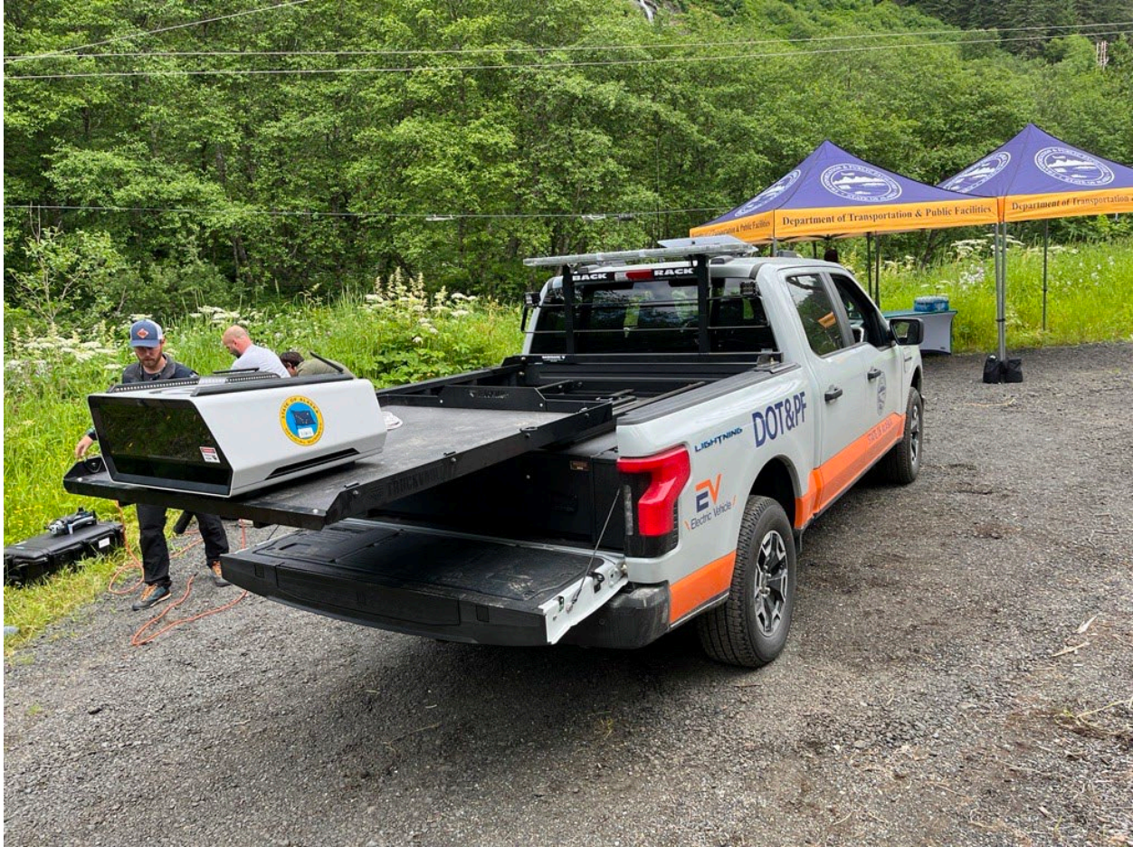
Figure 8. Alaska DOT&PF Electric Emergency Response Vehicle with UAS Dock System. (Source: FHWA)
