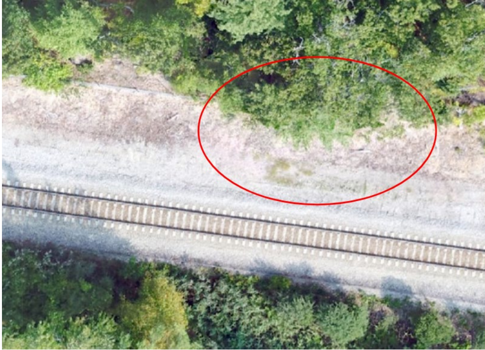
Figure 2. UAS Rail Inspection for Vegetation Encroachment. (Source: MassDOT)
