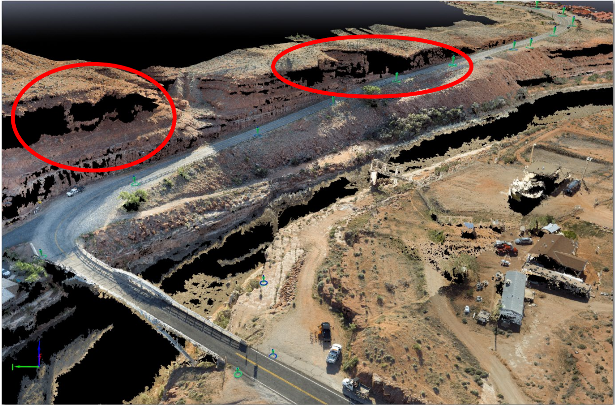
Figure 5. Missing Data with nadir angle 3D mapping (Photo courtesy of Utah DOT)
