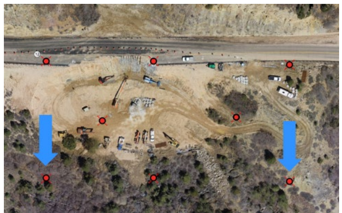
Figure 9. GCPs placement (Image courtesy of UDOT)
