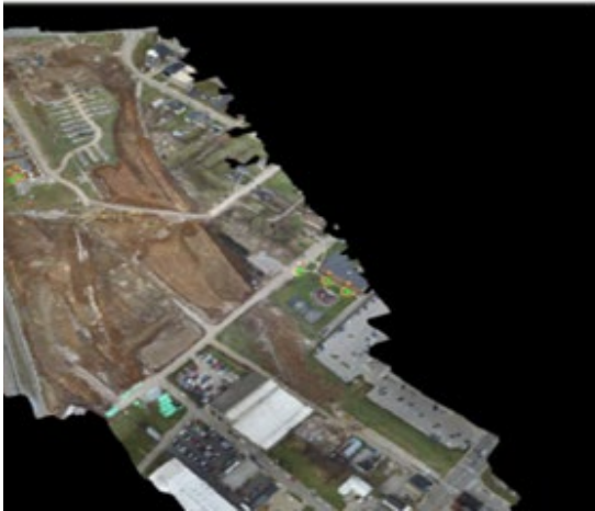
Figure 1. Dense point cloud developed using SfM (Image courtesy of Xi Wang, UKY)
