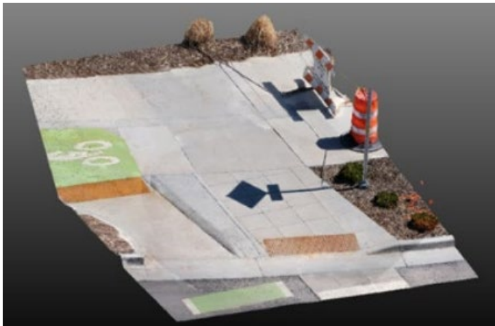
Figure 7. 3D Model of Pedestrian Ramp. Source: UDOT
